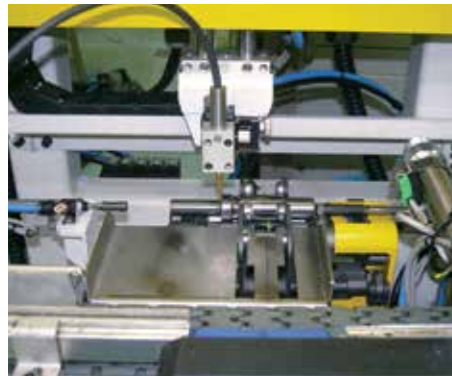
Bearing shaft ECT
