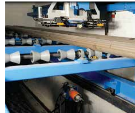
STS pipe digital RT (Triple FPD's)
