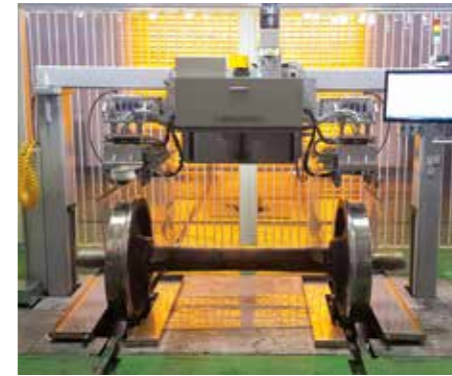
Train wheel & axle inspection
