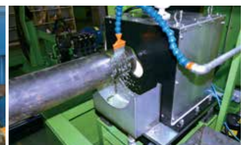
Surface crack inspection
