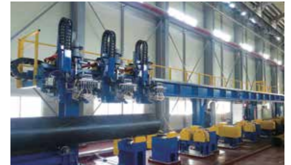
Triple heads conventional UT
