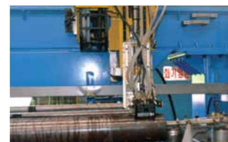
Internal/External crack inspection
