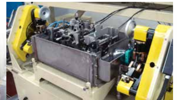
Half immersion UT (Special tube)
