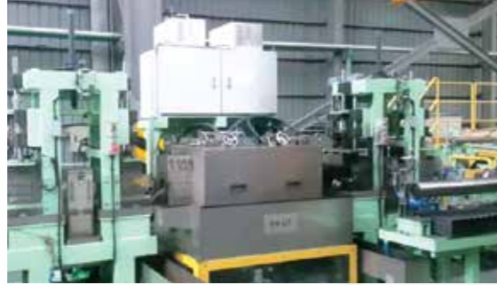
Immersion phased array UT
