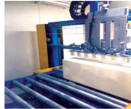
Non-contact air coupled UT
