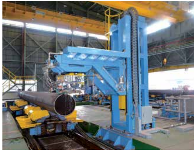
Pipe moving type (LSAW)
