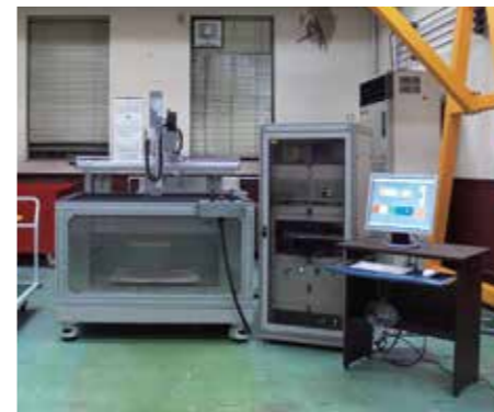
Immersion C-scan (HIC & cleanliness)
